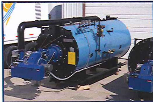
Fire Tube Boiler
